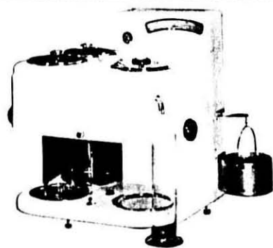
TYPE BL 95. For all types of Paste Goods, Flour and Semolina. Measures: (1) Cooking degree; (2) Volume of dry paste goods; (3) Volume of Cooked Paste Goods; (4) Increase in Volume during cooking process (water absorption); (5) Amount of sludge deposit left in cooking water. Extremely compact laboratory model. Operates electrically; thermostat-controlled.
